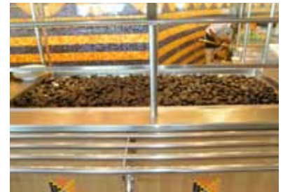
Chilled river rocks are used to keep food cold in buffets on Celebrity Cruises ships.
